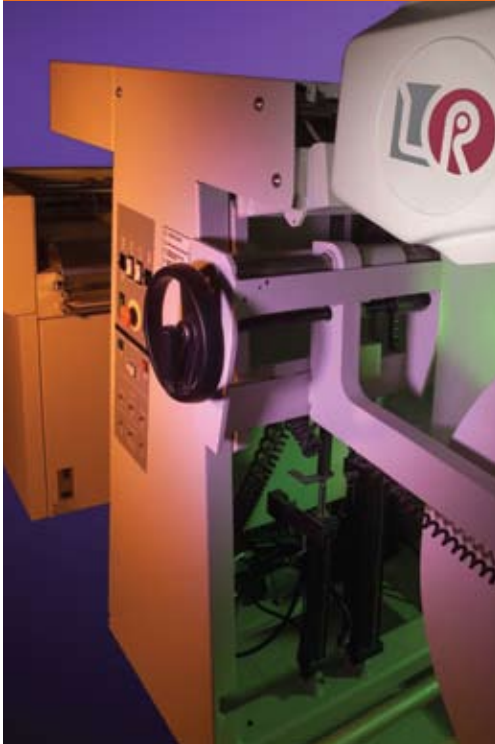
The DocuSheeter VP 5000 works in conjunction with the Océ VarioPrint 5000 digital printer and consists of an unwind, cutter and sheet transport.
